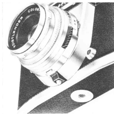
3-20. To remove lens, catch at base of camera is depressed while lens is turned to left.
